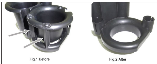
Illustration AF - Suzuki GSX-R 1000 2nd Air Funnel Removal.
